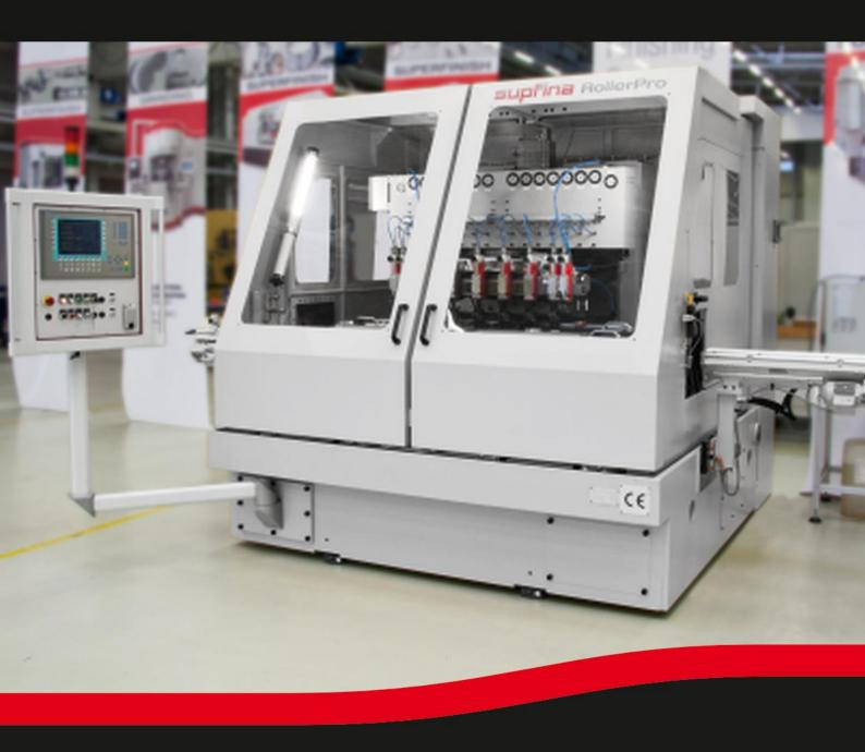
Superfinishing of cylindrical and tapered rollers
