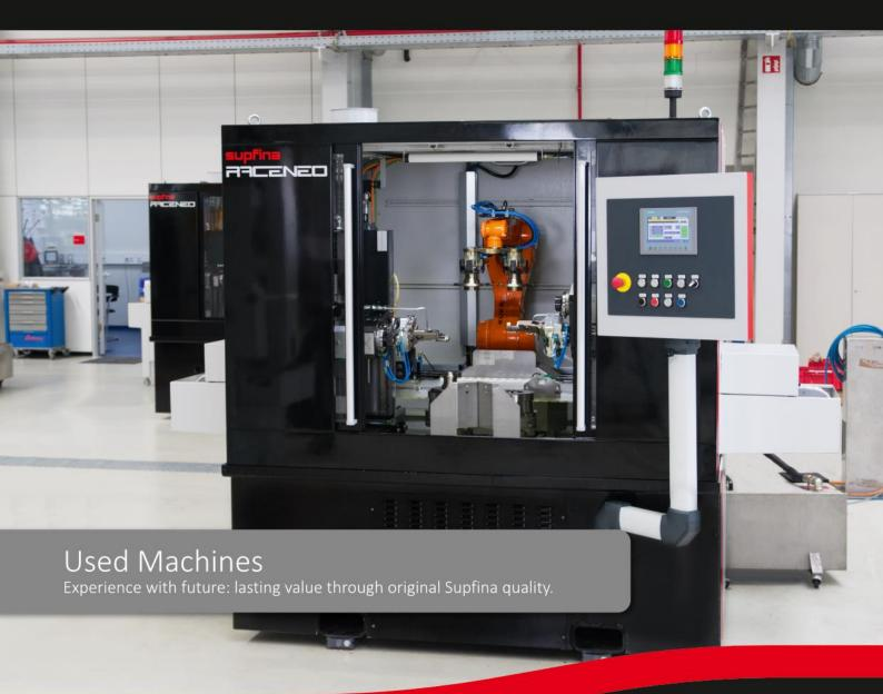
Superfinishing of raceways Inner and outer rings
